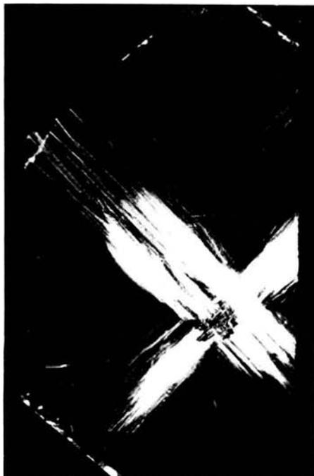
FIG. 6.8. X-ray topograph of triglycine sulphate crystal showing bundles of dislocations radiating from the seed (Vergnoux *et al.*, 1971).
