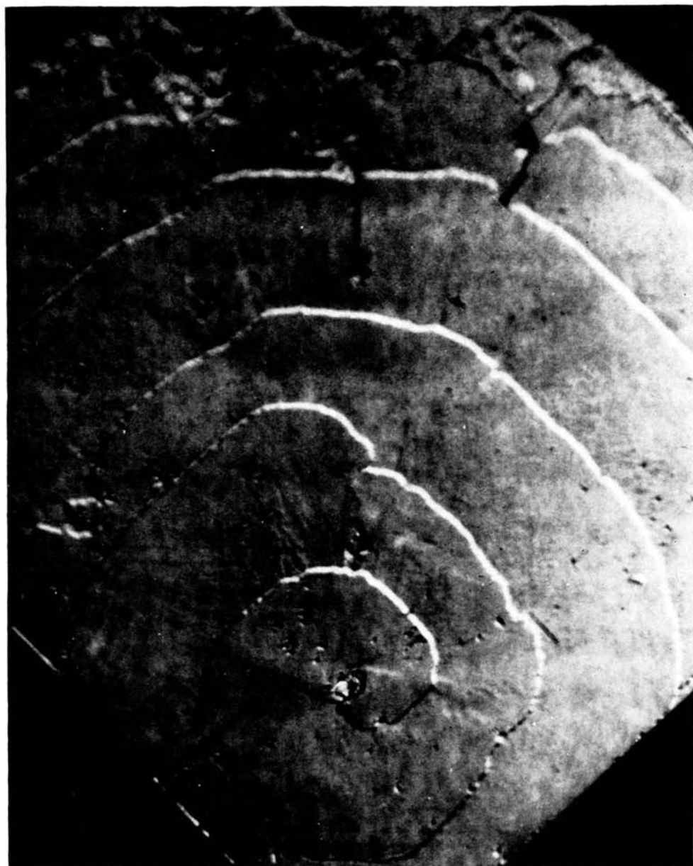
FIG. 7.51. Growth spiral on a (100) face of diamond grown in nickel (Strong and Hanneman, 1967).
