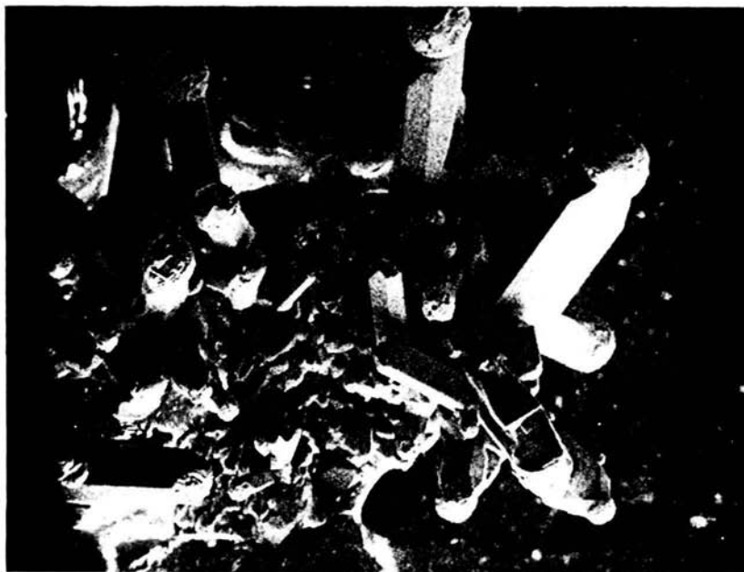
Fig. 7.21. VLS growth demonstrated by the solidified droplet at the end of \text{CaB}_6 whiskers (Rea and Kostiner, 1971).
